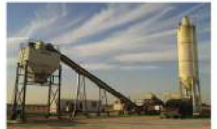
WET MIX MACADAM PLANT
