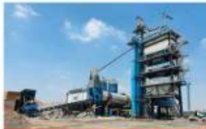
ASPHALT BATCH MIX PLANT
